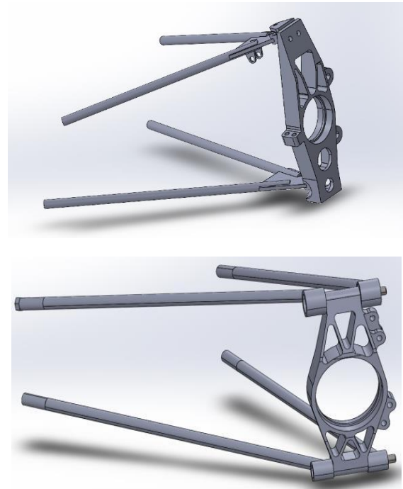
Figure 3- Assembly in SolidWorks
