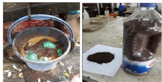
Fig-2: Adsorption process by tea leaves powder
