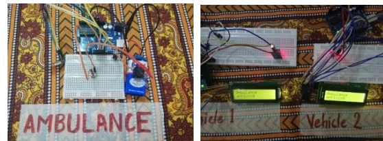
Fig -10 : (a) Ambulance node and (b) vehicle nodes showing ambulance arriving signal
