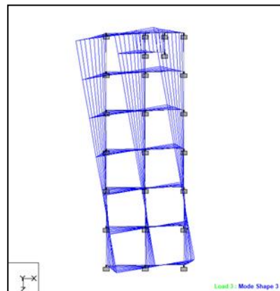
Fig-10: First torsional mode shape for model 2
