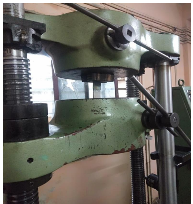
Fig-7: Tensile Test of Workpiece On UTM
