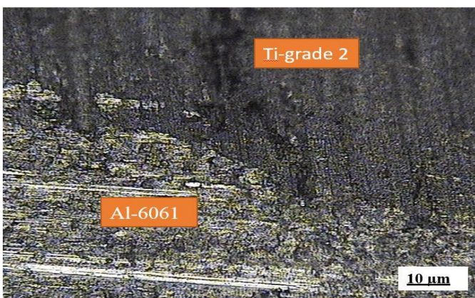
Fig-8: Metallurgical Bonding of Al-Ti
