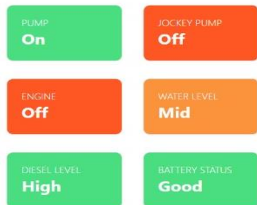
Figure 3.2: Overall System's health, important information about the pump, engine, water level, diesel level and battery status.
