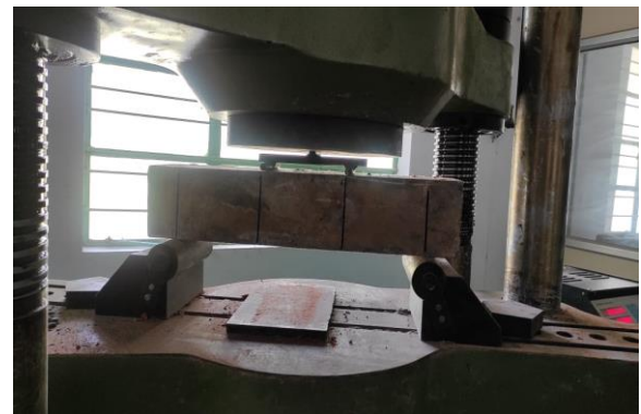
Figure-3: Testing of beam
