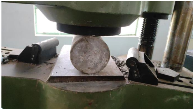
Figure-2 Testing of cylinder
