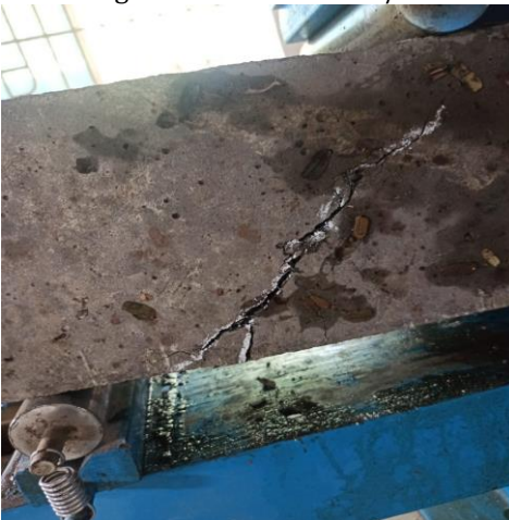
Fig -3: crack pattern of beam with steel fibre on full depth
