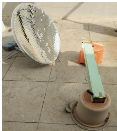
Fig-4: experimental setup for Analysis of efficiency of concentrator and mirror tube
