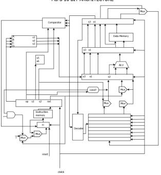
The execution of each instruction in a processor can be split up into a certain number of stages. The purpose of each stage is different for each processor design. The MIPS processor has 5 stages: Instruction Fetch, Instruction Decode, Execution stage, Memory stage, and Write Back stage.
