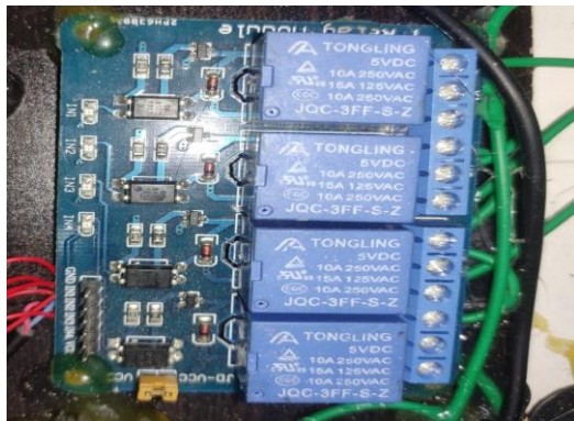
Fig-6: RELAY DRIVER CIRCUIT
