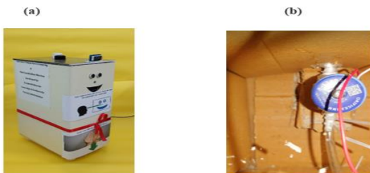
Fig. 12(a) – Third model of machine with an additional 7 segment display module on top. (b) The attachment of solenoid valve below the sanitizer tank.
