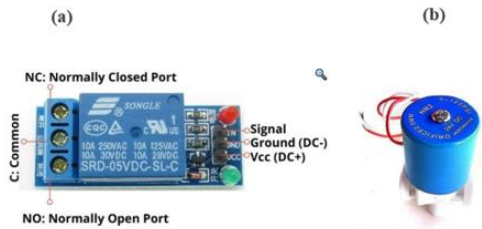
Fig. 5. (a) Relay module used for operating solenoid valve. (b) Solenoid Valve
