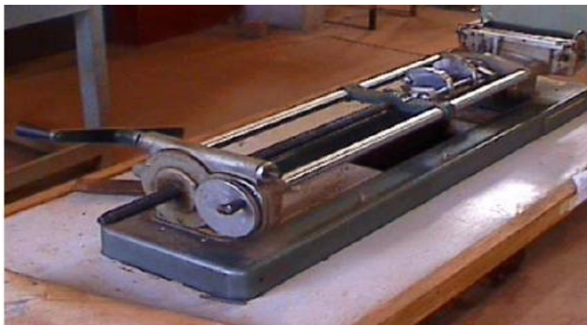
Figure 7: Hounsfield Monsanto Tensometer (Model no: S/N 8889)
