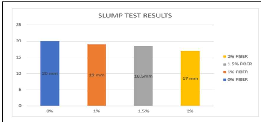
Figure 3 Slump test results for the various percentage of waste steel fiber.
