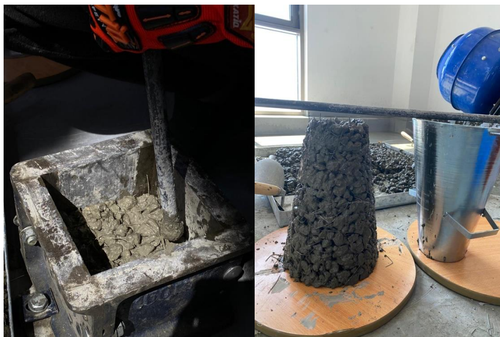
Figure 2 Tampering of concrete with slump test performed during the concrete casting.
