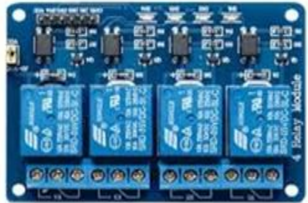
Fig. 3- Four channel relay unit
