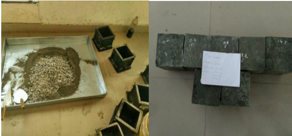
Figure 3.5 Mixing and Casted specimens
