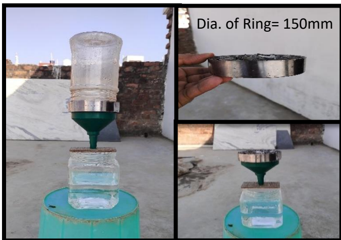
Water Permeability Test
