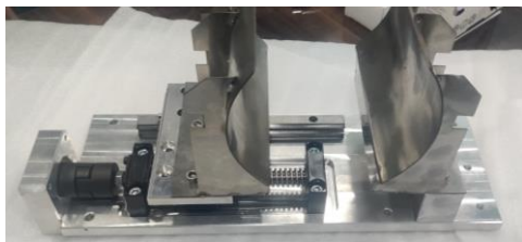
Fig - 5: Lead Screw Ambu Bag Compression Mechanism [Courtesy Robonist Tech Solutions PVT.LTD]
