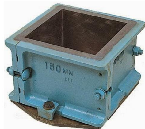
Fig -1: Cube Specimen of size 150mm X 150mm X 150mm
