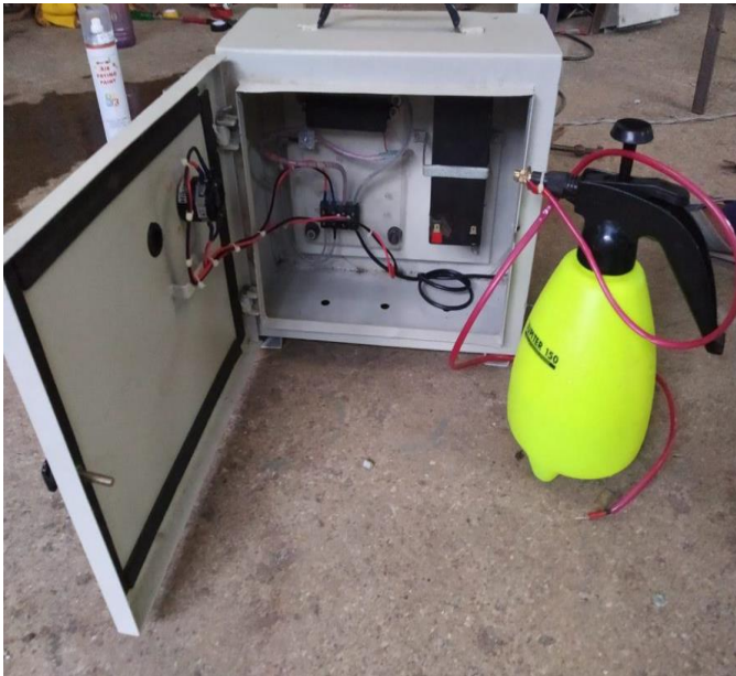
Figure 3 Complete setup of Electrostatic Spraying system
