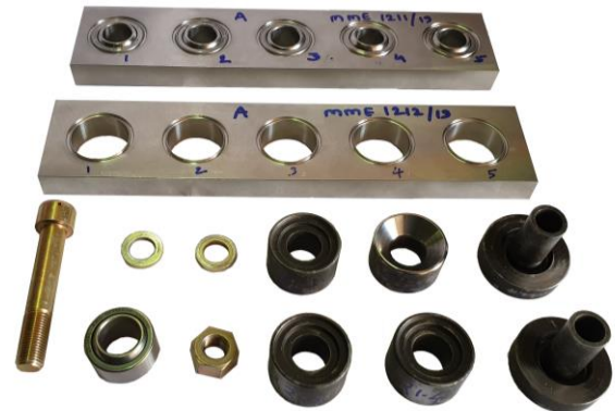
Fig-13: Staked interfaces, Plate, Staking Tools, Fastener set and Spherical bearing
