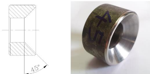
Fig-9: Staking tool with angle 45°
