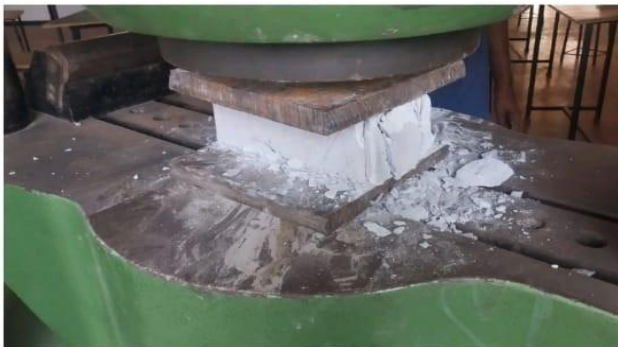
Fig 2 – Compressive strength test
