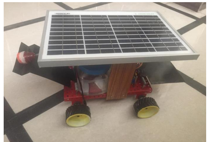
Fig-4: Snap shot of Prototype model with solar panel
