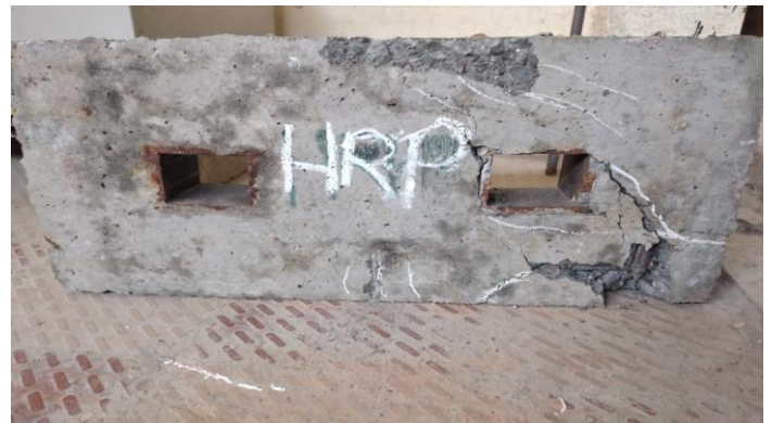
n) HRP beam after Testing
