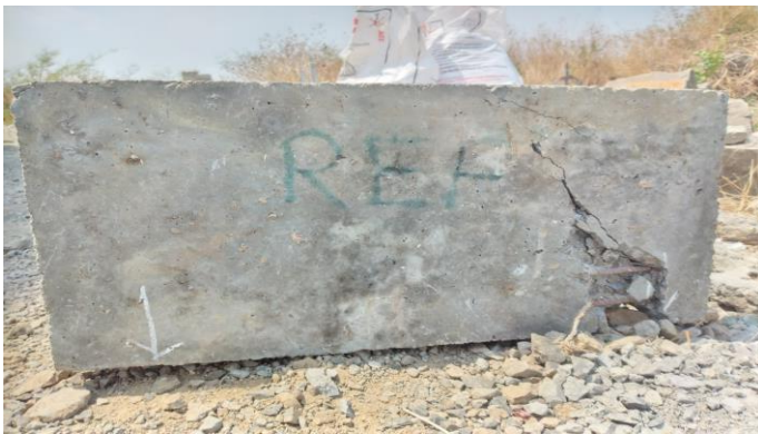
l) REF beam after testing
