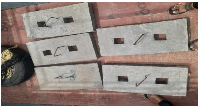
f) Specimens of Deep beam after 28 days curing
