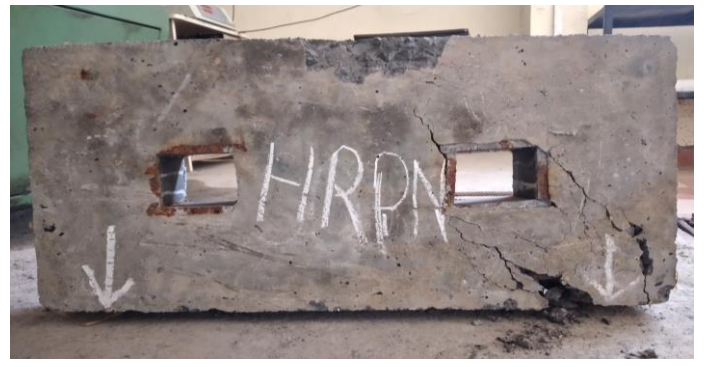
o) HRPN beam after testing
