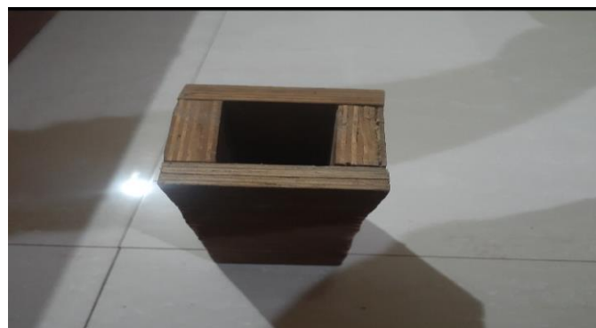
g) Wooden prism used to make openings
