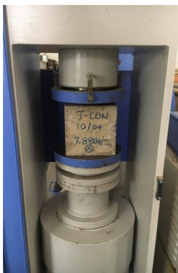
Fig -3: Compressive strength for cube
