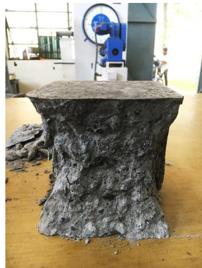
Fig -4: Tested cube specimen
