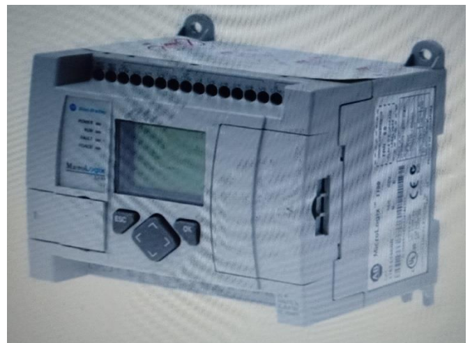
Fig. ALLEN BRADLEY PLC (micrologix 1100)
