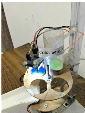
Fig - 13: Color sensor sensing blue object
