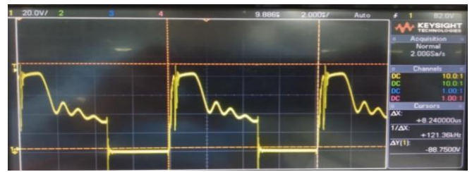
Fig -7: Drain Source Voltage across main MOSFET
