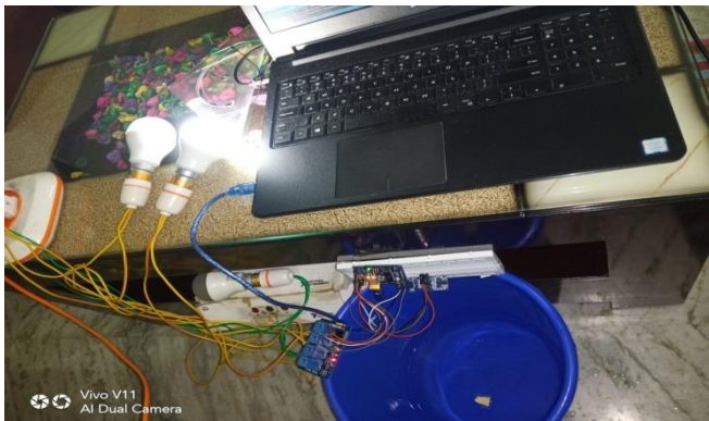
Fig -12: Indicating water is at medium level
