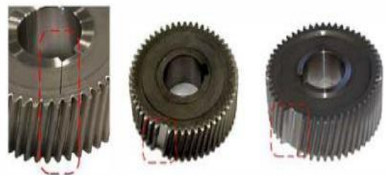
Fig. 7: Gears with tooth defects
