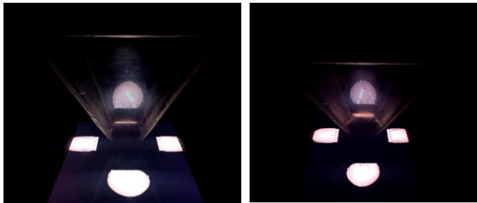
Fig -18: Image displaying the Pyramid Hologram Prototype via iPad Screen
