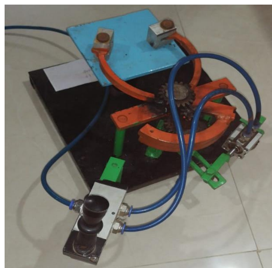
Fig -2: manufactured pneumatic self centering clamp
