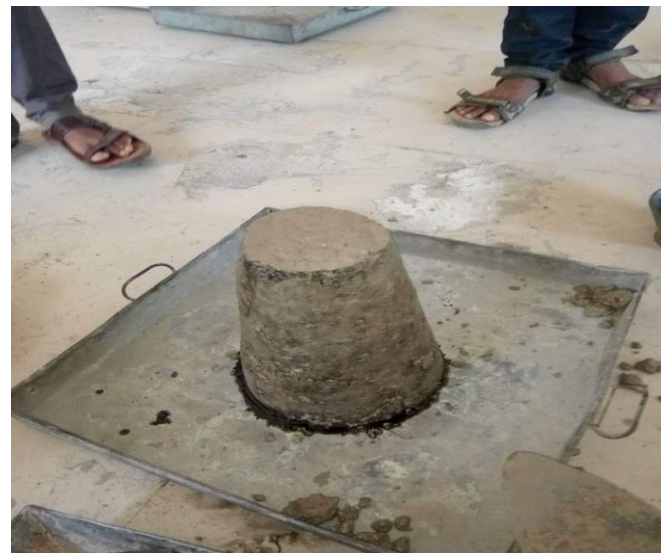
Fig-1: Slump cone Test
