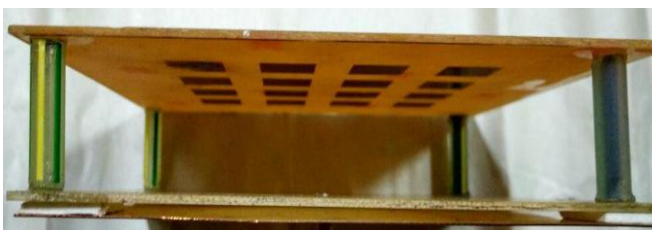
Fig.7. Fabricated Antenna structure
