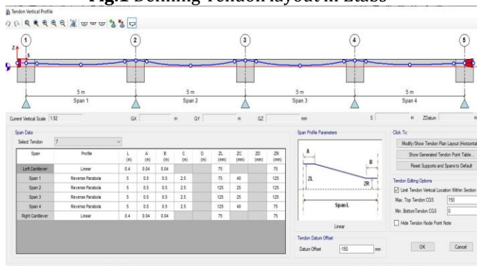
Fig.2 Distributed Tendon Profile
