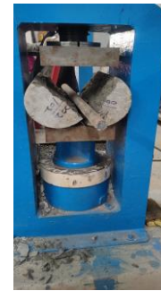
Fig -2: Split Tensile Strength Test.
