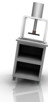
Fig -5.2: 3D View of the Pneumatic Sheet Metal Cutter.
