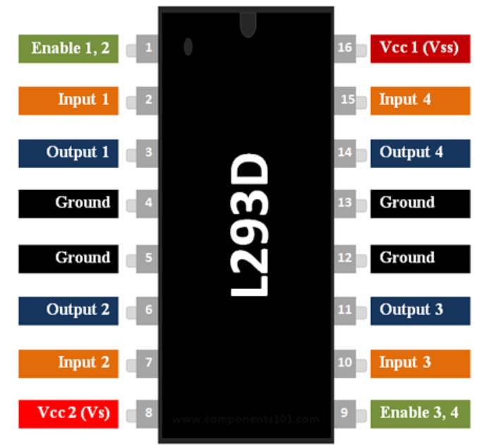
Figure -22: Pin Diagram of L293D
