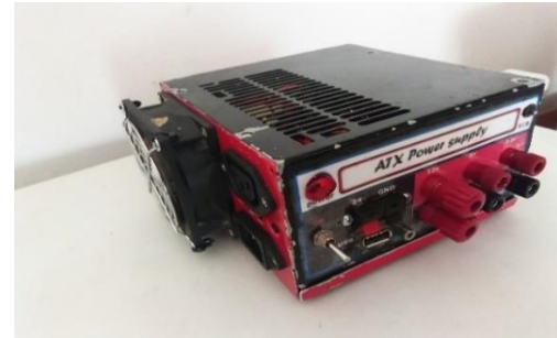
Figure 1811: NC bench power supply from the PC power supply.
