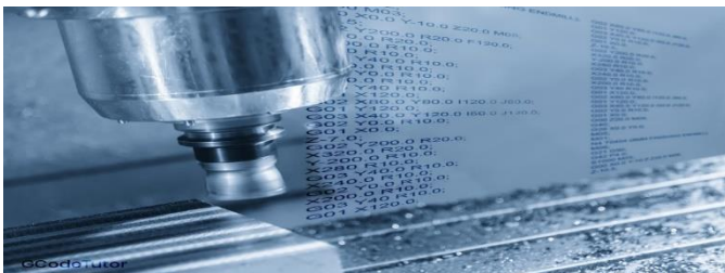
Figure 2: G-Codes and M-codes from a computer used as instructions to a milling machine [6]
