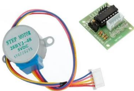
Figure 105: ULN2003 Driver Board and 5 wire 5v 4 phase 28BYJ-48 unipolar stepper motor [23].
