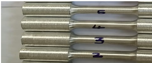
Fig 4.1 Tensile Test Specimens
