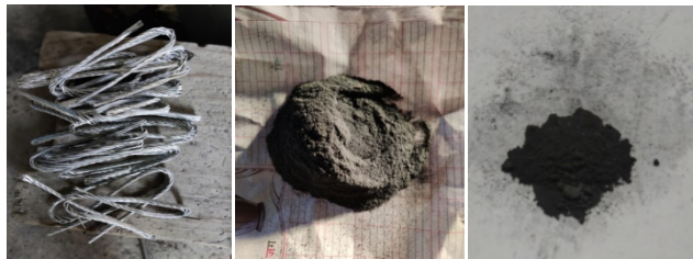
Fig1.1 Samples of Aluminum pieces, TiB_2 and Gr Powder
