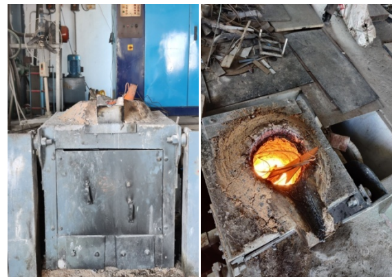
Fig 3.1 Induction Furnace Stir casting
