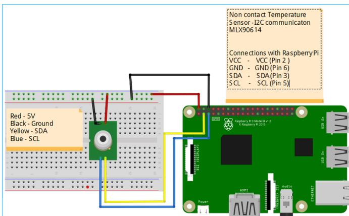
Figure 1. Circuit Diagram
