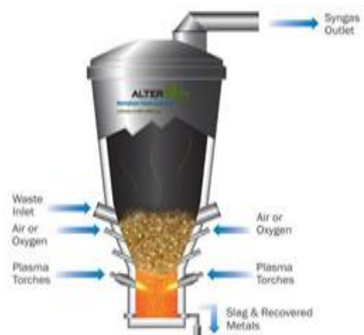
Fig. 3. Waste processing in gasifier
