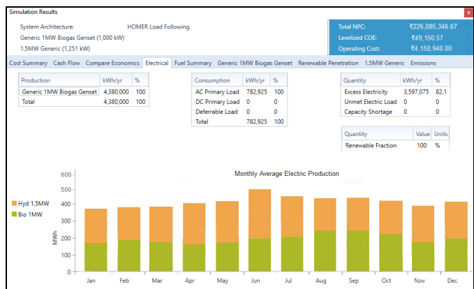
Figure 7. Monthly average electricity generation by the Biogas – Mini Hydro Power system
