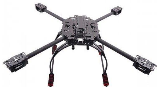
Fig-14 650 mm CF Quadcopter frame
