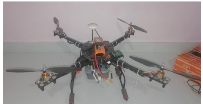
Fig-15 Assembled Quadcopter with Paint Dispersion Mechanism
