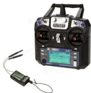
Fig-10 Fly sky i6 2.4 6CH Transmitter and FS-i6 Receiver
