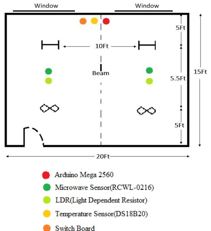
Fig -2: Room Plan with Sensor Sectioning
