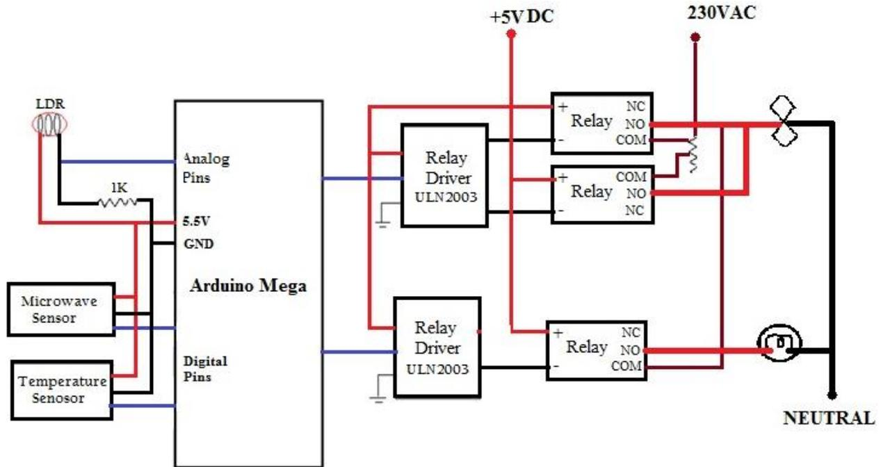
Fig -4: Main proposed circuit diagram
