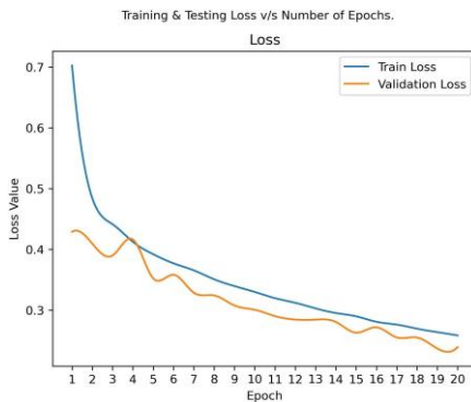
Figure 8. The transition graph of training loss with increasing number of epochs in MesoNet
