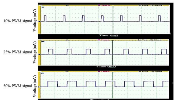
Fig -6: PWM Signals during Dimming Test
