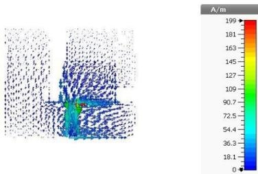
**Fig.3d.** Surface current at 3.853 GHz frequency.
