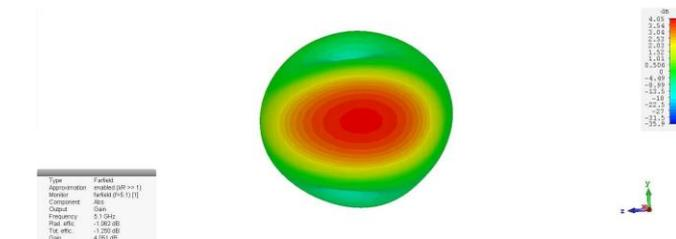
**Fig.4.** Gain at 5.1 GHz frequency.
