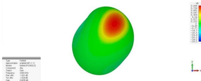
**Fig.3e.** Gain at 3.853 GHz.
