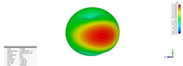
**Fig.5.** Gain at 5.3 GHz broadband frequency.
