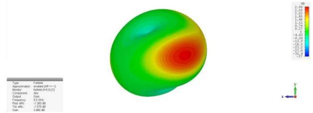
**Fig.6.** Gain at 5.5 GHz broadband frequency.
