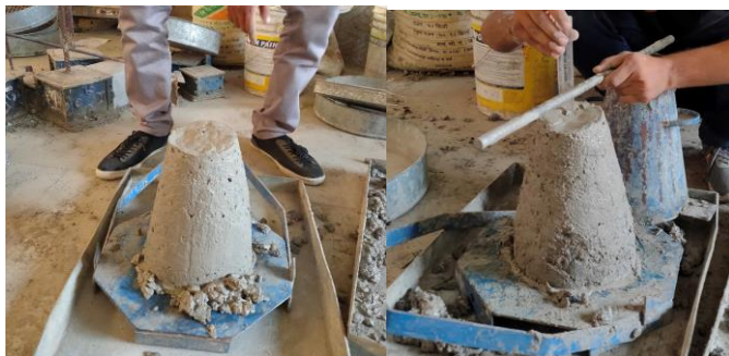
Fig -3: Slump Cone Test
