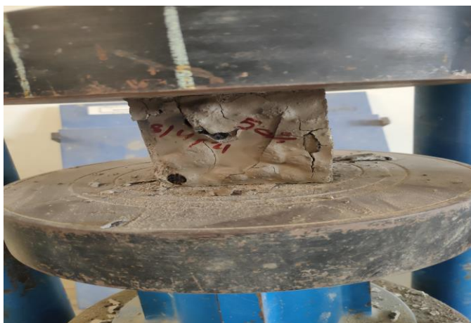
Fig -4: Compressive Strength Test
