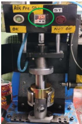
Fig.5: Leak Test Setup
